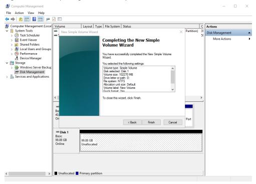
Figure 2-22 Completing the New Simple Volume Wizard
