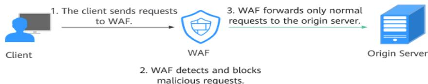
The process of forwarding traffic from WAF to origin servers is called back-to-source. WAF uses back-to-source IP addresses to send client requests to the origin server. When a website is connected to WAF, the destination IP addresses to the client are the IP addresses of WAF, so that the origin server IP address is invisible to the client.
